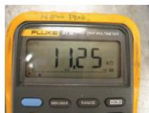
Measuring Scroll NTC Resistance
