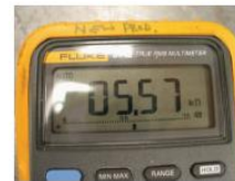
Measuring Motor NTC Resistance
