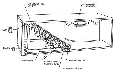
Fig. 5 - Conversion for Horizontal Right Applications - Slope Coil
