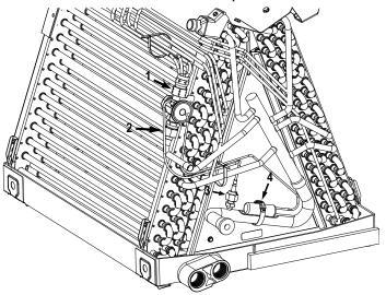
Fig. 16 - Mechanical TXV Removal
