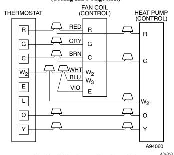
Fig. 12 – Wiring Layout Heat Pump Unit (Cooling and 2-Stage Heat with No Outdoor Thermostat)
