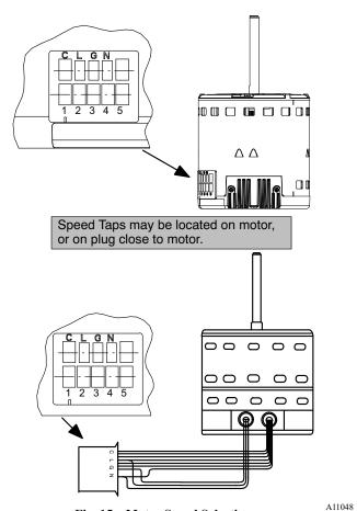
Fig. 15 - Motor Speed Selection
