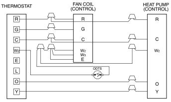
Fig. 13 – Wiring Layout Heat Pump Unit (Cooling and 2-Stage Heat for Manufactured Housing)
