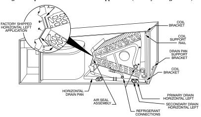
Fig. 4 – A-Coil in Horizontal Left Application (Factory Configuration)
