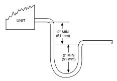
Fig. 17 – Recommended Condensate Trap
