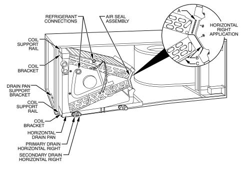
Fig. 6 - Conversion for Horizontal Right Applications - A-Coil
