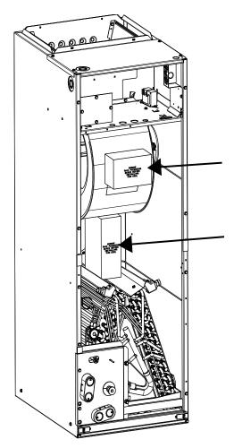
Fig. 1 – Remove Shipping Blocks
