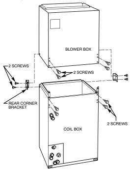
Fig. 7 - Removal of Brackets on Modular Unit
