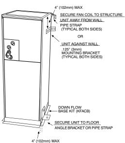
$\textbf{Fig. 9-Mobile Home or Manufactured Housing Applications}^{A07567}$
