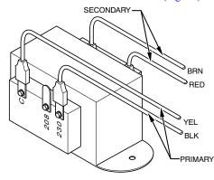
Fig. 14 – Transformer Connections
