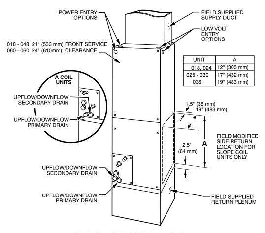
Fig. 2 - Slope Coil Unit in Upflow Application
