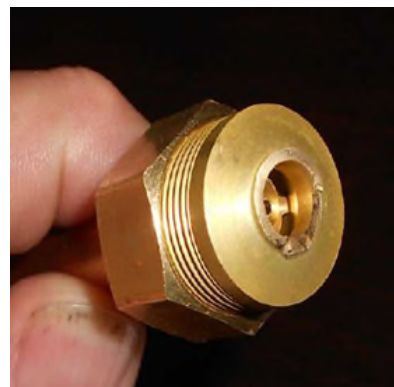
Service valve connector failure (Over torqued) with HP adapter.
