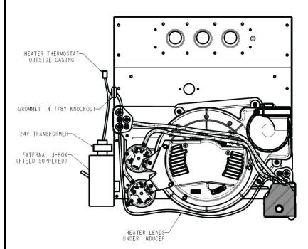
The trap heater kit includes a completely new trap with the heating pad affixed to it to prevent freezing of condensate in the trap. The kit also includes a step-down transformer that provides the 24V required for the heating pad, and an in-line thermostat to turn on the heating pad when ambient temperatures reach 35 degrees.
