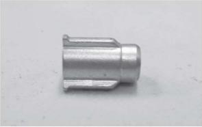
5.) Clean all debris found in the piston body with a Q-tip then clean the piston with a rag. **Note:** The injection of Zerol Ice additive has not been found to be an effective way clean the debris from the piston/body and allow the piston to seat. It is however a very good product for manually cleaning the parts.
