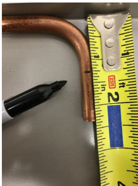
3. Measure 1 1/4" to obtain cut point.
