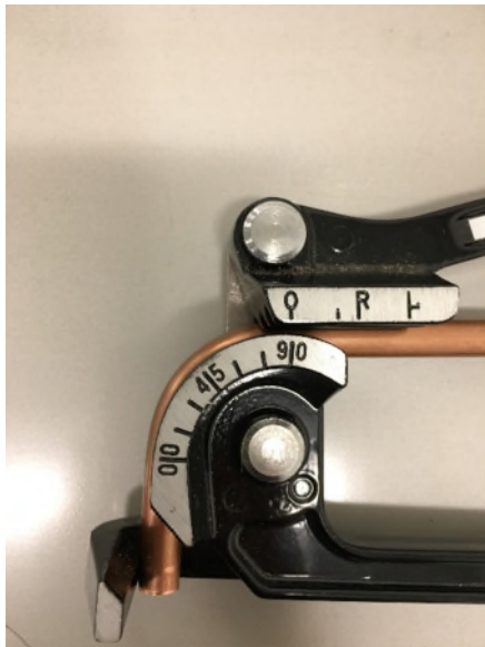
2. 90 degree bend in the end of the 3/8" line set.
